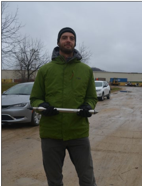
Greg Wachman, senior geotechnical engineer in engineering and construction division, holds the cone for a cone penetrometer test, in Arcadia, Wisconsin, Nov. 12. USACE photo by Melanie Peterson
